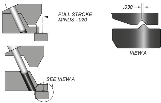
**NOTE:** Set angle pin to release .020 from full stroke. Striker will snap to full stroke to assure re-entry clearance of angle pin.
