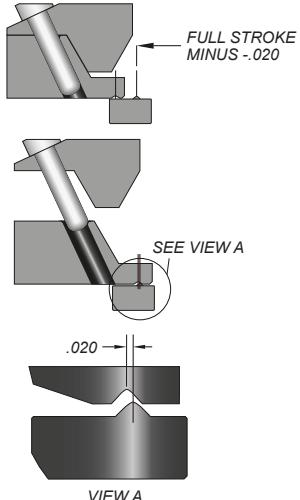
**NOTE:** Set angle pin to release .020 from full stroke. Striker will snap to full stroke to assure re-entry clearance of angle pin.
