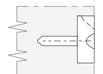
The latch is usually mounted into the slide because of normal space limitations and requirements. This is not a rule though, and the designer may locate the various components to best suit the application.
